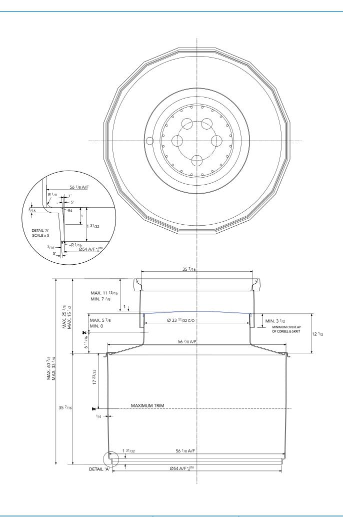
$57^\circ$  dia. FRP sump with  $54^\circ$  tank collar ring connection, corbel, skirt, internal lid,  $36^\circ$  dia. flat sealed cover and composite frame.
