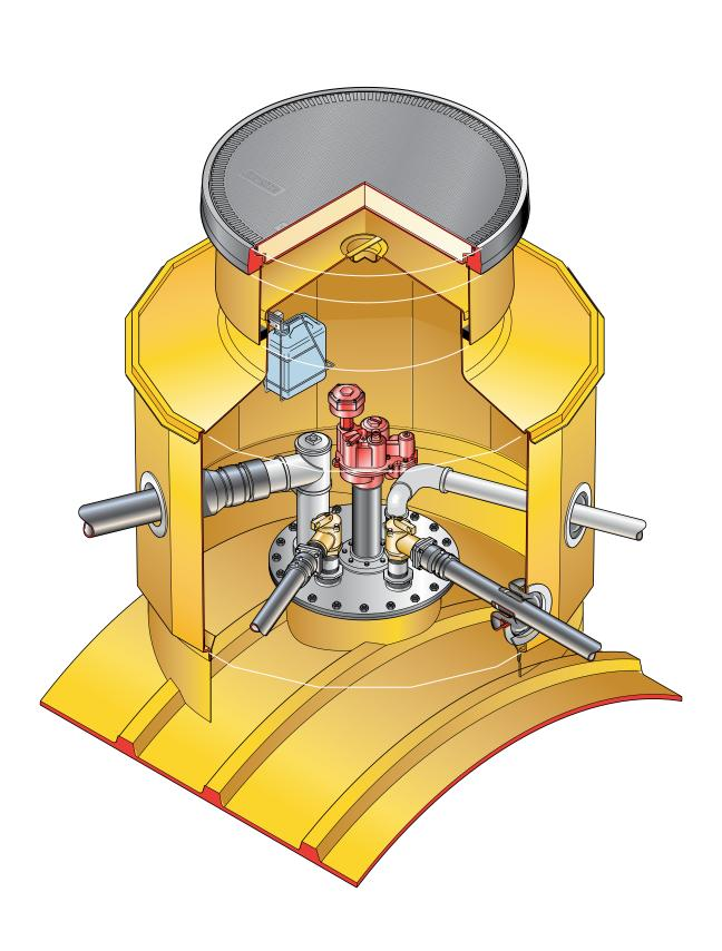
$57^\circ$  dia. FRP sump with  $54^\circ$  tank collar ring connection, corbel, skirt, internal lid,  $36^\circ$  dia. flat sealed cover and composite frame.
