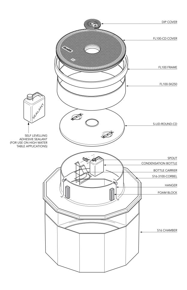
59" diameter 12 sided sump with reverse flange, corbel, adjustable height skirt, internal lid with dip tube hole, round 40" flat sealed cover and frame with central dip cover.
