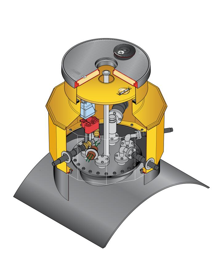
59" diameter 12 sided sump with reverse flange, corbel, adjustable height skirt, internal lid with dip tube hole, round 40" flat sealed cover and frame with central dip cover.
