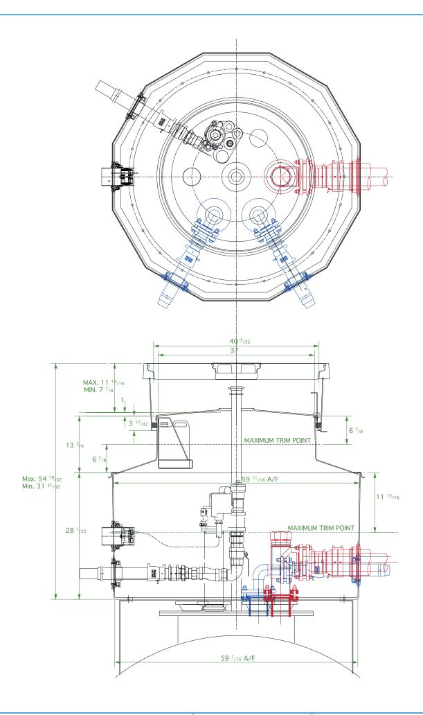
59" diameter 12 sided sump with reverse flange, corbel, adjustable height skirt, internal lid with dip tube hole, round 40" flat sealed cover and frame with central dip cover.
