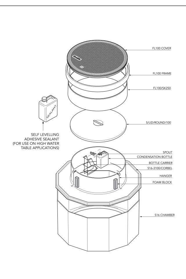
59" diameter 12 sided sump with reverse flange, corbel, adjustable height skirt, internal lid with dip tube hole, and round 40" flat sealed cover and frame.
