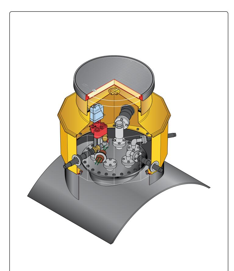
59" diameter 12 sided sump with reverse flange, corbel, adjustable height skirt, internal lid with dip tube hole, and round 40" flat sealed cover and frame.
