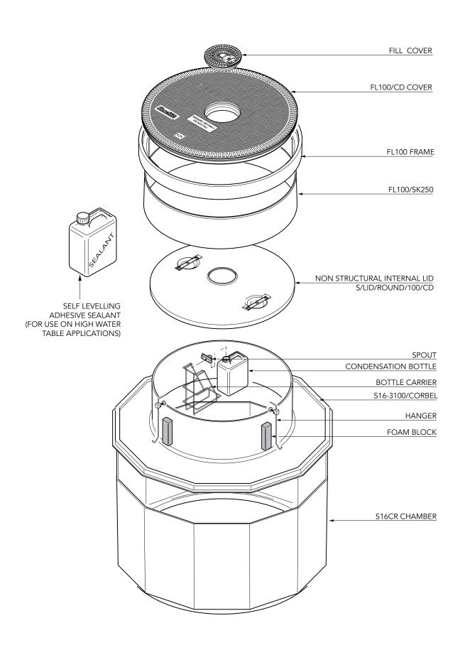
59 1/16" dia twelve sided sump with collar ring base. corbel, skirt, non structural internal lid with dipstick hole. 42" dia flat sealed black cover with central sealed cover and frame. Designed for a remote fill line with a central dip.
