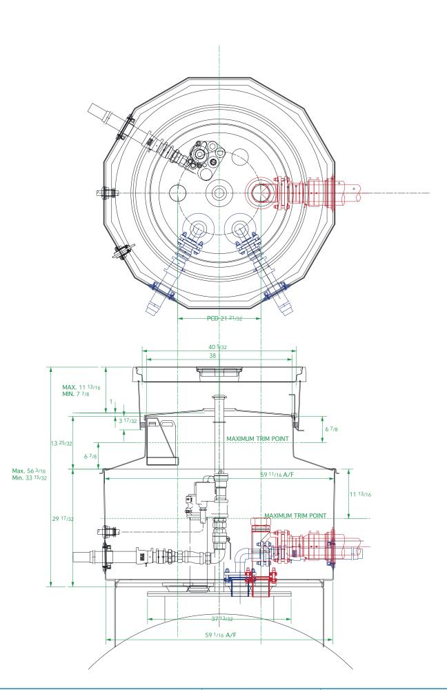
59 1/16" dia twelve sided sump with collar ring base. corbel, skirt, non structural internal lid with dipstick hole. 42" dia flat sealed black cover with central sealed cover and frame. Designed for a remote fill line with a central dip.
