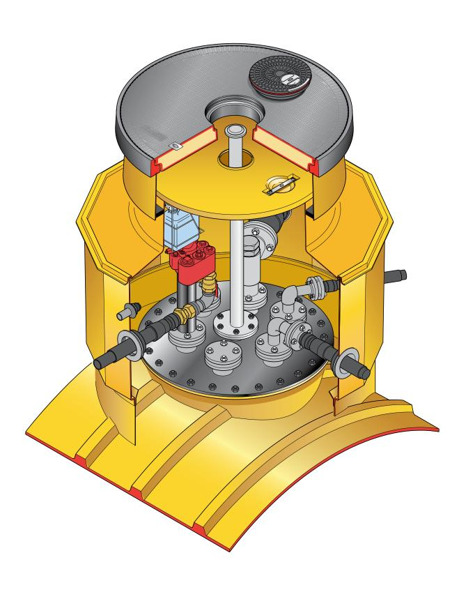
59 1/16" dia twelve sided sump with collar ring base. corbel, skirt, non structural internal lid with dipstick hole. 42" dia flat sealed black cover with central sealed cover and frame. Designed for a remote fill line with a central dip.
