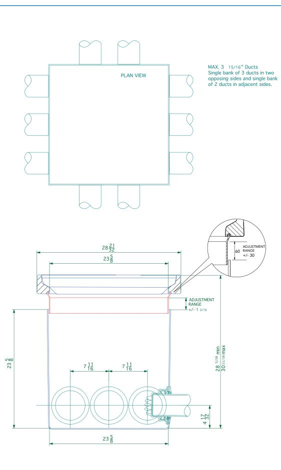
Electrical Drawpit - 23 5/8" cubed GRP chamber with a 4 11/32" deep GRP skirt and 23 5/8" square flat sealaed cover.
