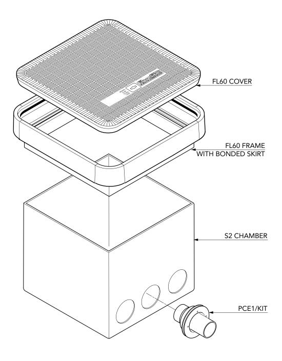
Electrical Drawpit - 23 5/8" cubed GRP chamber with a 4 11/32" deep GRP skirt and 23 5/8" square flat sealaed cover.
