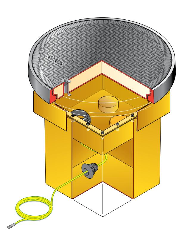
19 9/32" square x 30 5/16" deep offset fill chamber system with adjustable skirt, spill container, 1/2 tin of sealant and FL760 flat sealed cover with composite frame. Includes inspection port cap, pipe entry and penetration fitting for grounding connection. For 1 fill.
