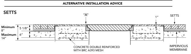
19 9/32" square x 30 5/16" deep offset fill chamber system with adjustable skirt, spill container, 1/2 tin of sealant and FL760 flat sealed cover with composite frame. Includes inspection port cap, pipe entry and penetration fitting for grounding connection. For 1 fill.
