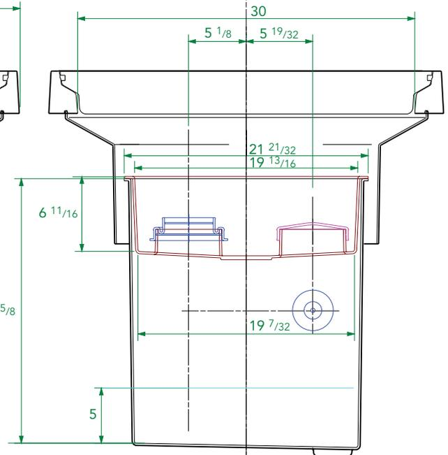
20" square x 24" deep GRP solid base sump, GRP spill container, GRP skirt, 30" dia flat sealed cover and frame. 1/2 tin sealant. 2 Fills.
