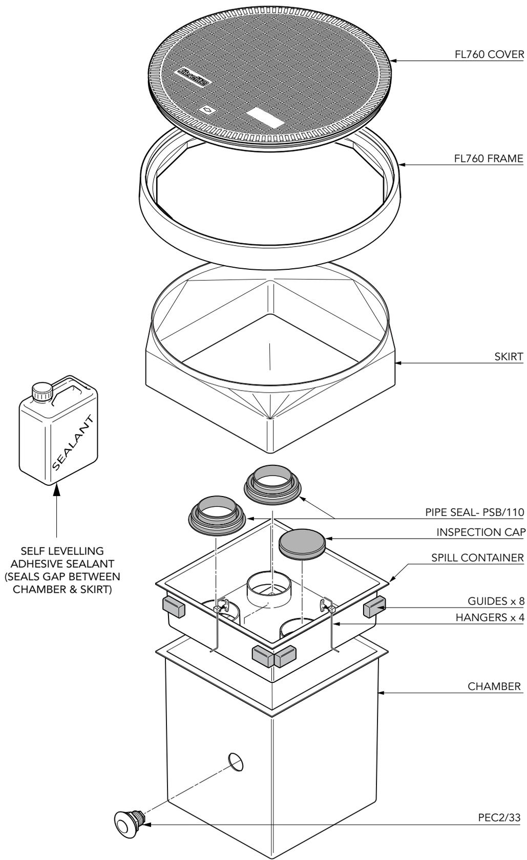
20" square x 24" deep GRP solid base sump, GRP spill container, GRP skirt, 30" dia flat sealed cover and frame. ½ tin sealant. 2 Fills.
