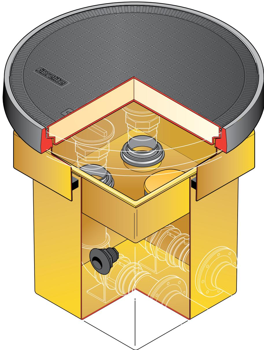
20" square x 24" deep GRP solid base sump, GRP spill container, GRP skirt, 30" dia flat sealed cover and frame. 1/2 tin sealant. 2 Fills.
