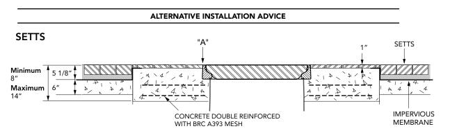
19 9/32" square x 30 5/16" deep offset fill chamber system with adjustable skirt, spill container, 1/2 tin of sealant and FL760 flat sealed cover with composite frame. Includes inspection port cap, pipe entry and penetration fitting for grounding connection. Includes preinstalled KPS pipework for 1 fill.
