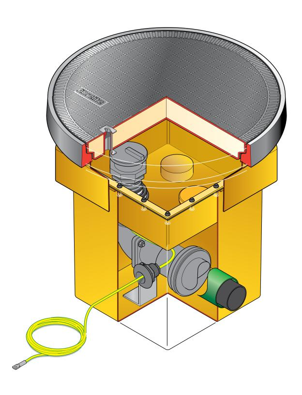
19 9/32" square x 30 5/16" deep offset fill chamber system with adjustable skirt, spill container, 1/2 tin of sealant and FL760 flat sealed cover with composite frame. Includes inspection port cap, pipe entry and penetration fitting for grounding connection. Includes preinstalled KPS pipework for 1 fill.
