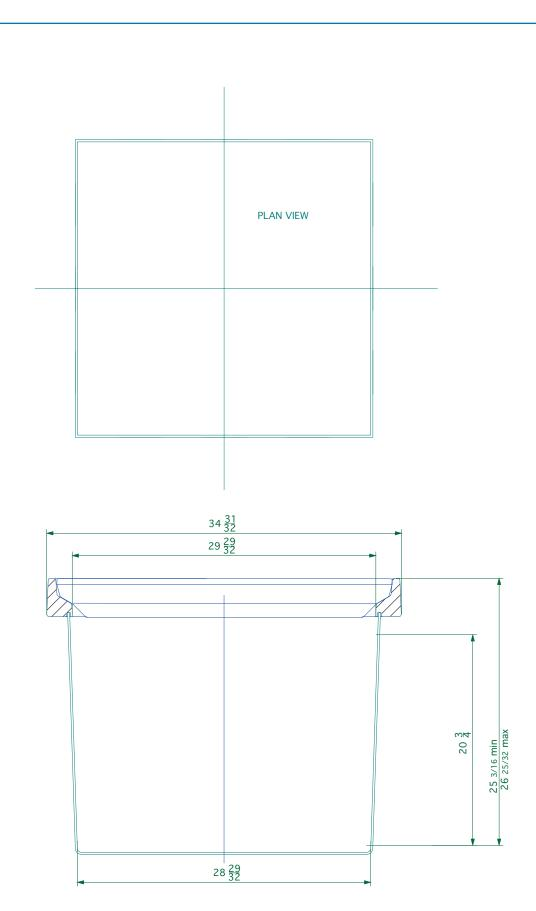
Electrical Drawpit 29 15/16" square x 23 5/8" deep solid base chamber with a square 29 15/16" flat sealed cover.a
