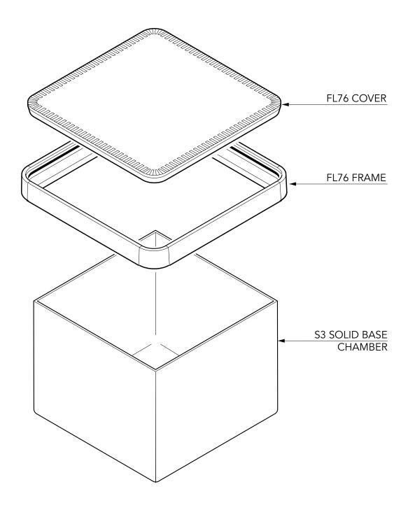
Electrical Drawpit 29 15/16" square x 23 5/8" deep solid base chamber with a square 29 15/16" flat sealed cover.a
