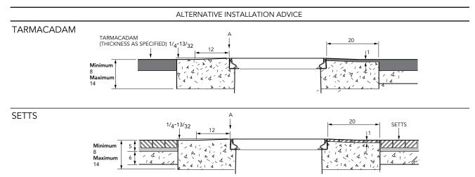
Electrical Drawpit 29 15/16" square x 23 5/8" deep solid base chamber with a square 29 15/16" flat sealed cover.a
