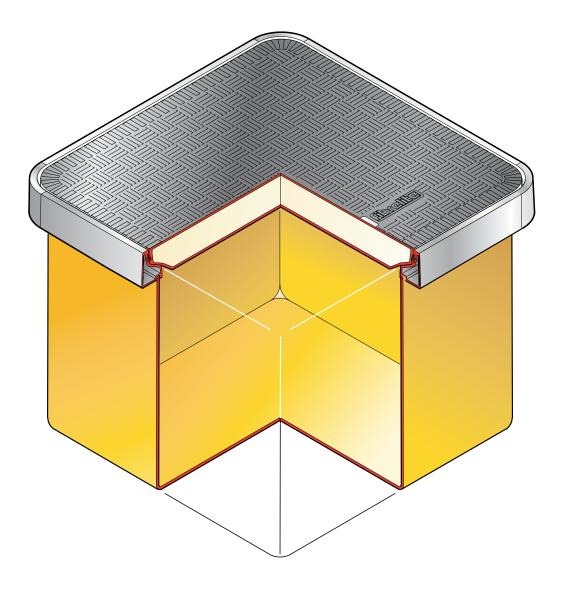
Electrical Drawpit 29 15/16" square x 23 5/8" deep solid base chamber with a square 29 15/16" flat sealed cover.a
