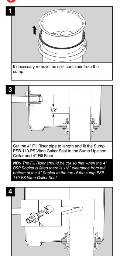
Fit the 1/2 BSP Cone Faced Adaptor to the welded 1/2" BSP Socket welded on the 4" BSP Socket. Then fit the 4" BSP Socket to the 4"Fill Riser.
