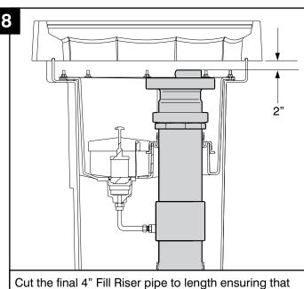
when the Fill Cap and Adaptor is fitted the top of the cap is 2" below the bottom of the FL180 Access Cover.
