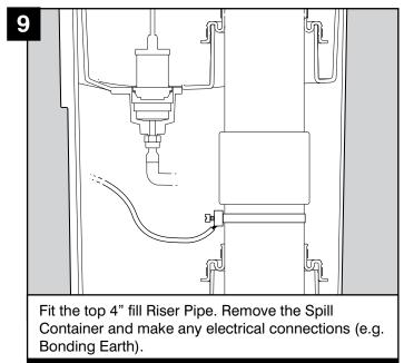
**NB:-** At this stage the Fill Riser can be plugged off and the system vacuum tested. The system must only be tested at 24".
