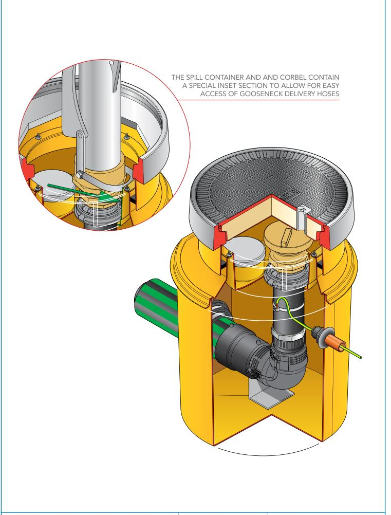
Secondary contained remote fill sump. 23" dia. x 25" deep solid base sump with a sealed secondary spill container. 18" dia flat sealed cover and frame. Sealkits included.
