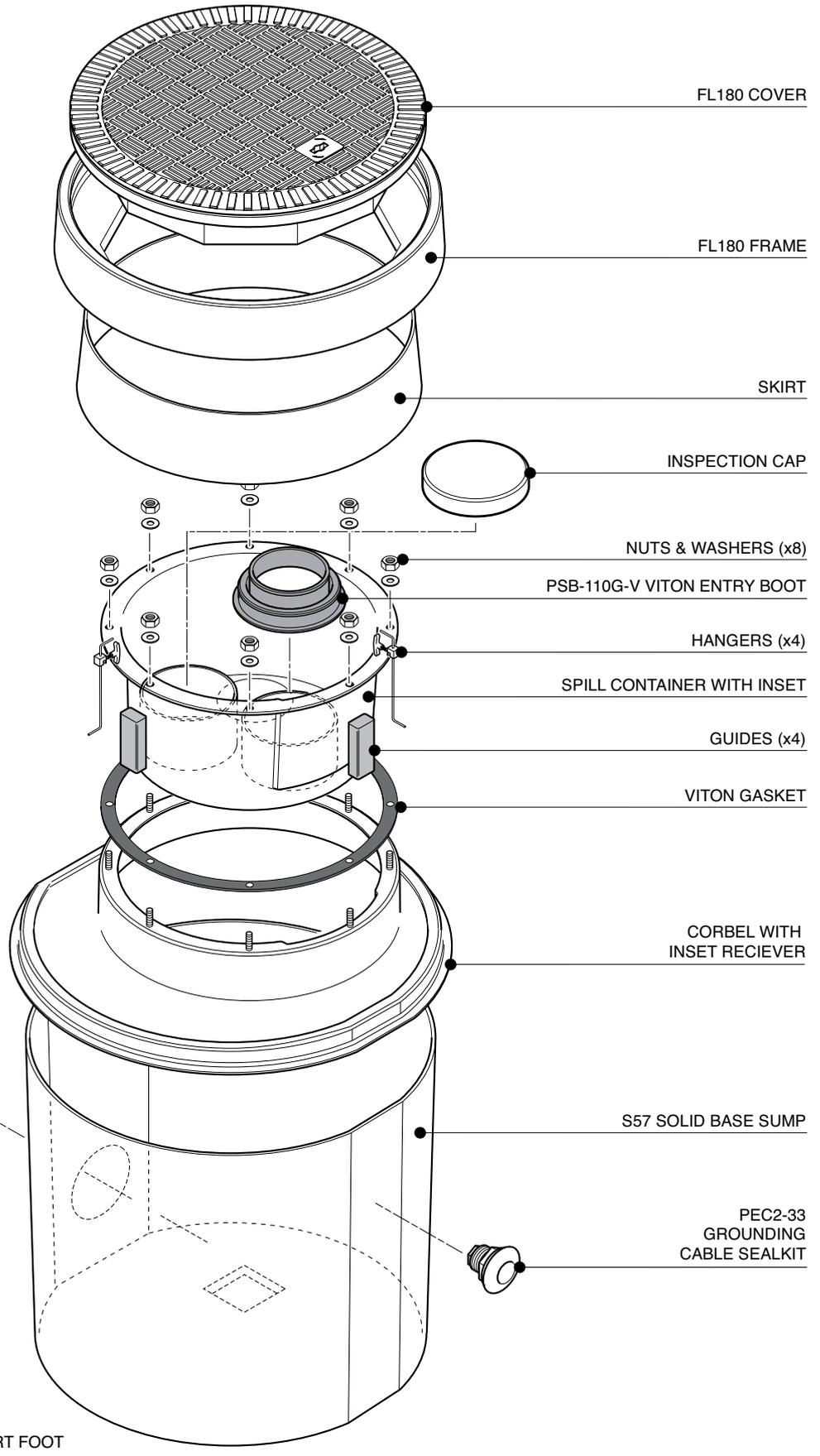
Secondary contained remote fill sump. 23" dia. x 25" deep solid base sump and a sealed secondary spill container. 18" dia flat sealed cover and frame. Includes PSB-110-PS 4 5/16" dia. spill tray fill riser sealkit and grounding cable sealkit.
