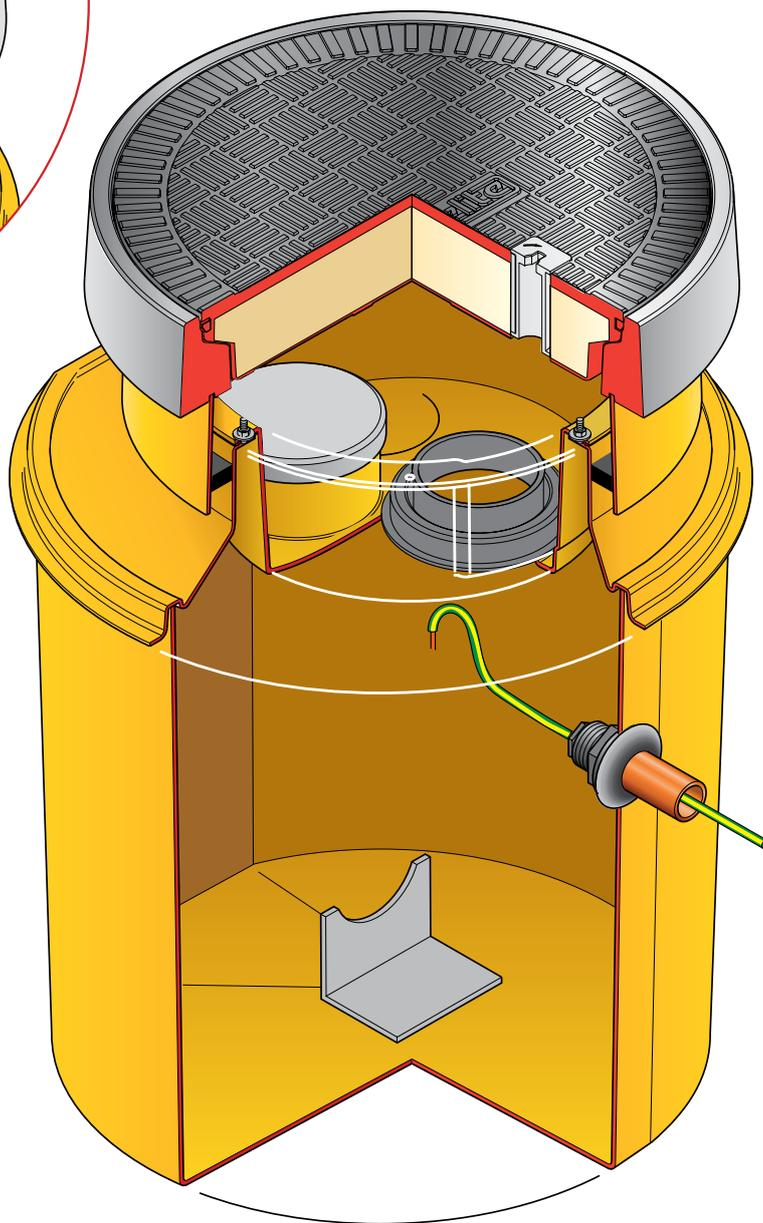
Secondary contained remote fill sump. 23" dia. x 25" deep solid base sump and a sealed secondary spill container. 18" dia flat sealed cover and frame. Includes PSB-110-PS 4 5/16" dia. spill tray fill riser sealkit and grounding cable sealkit.
