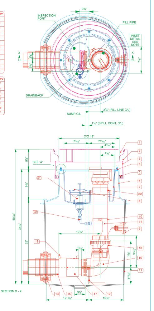
Secondary contained remote fill sump. 23" dia. x 25" deep solid base sump with a sealed secondary spill container with integrated drainback system. 18" dia flat sealed cover and frame. Sealkits included.
