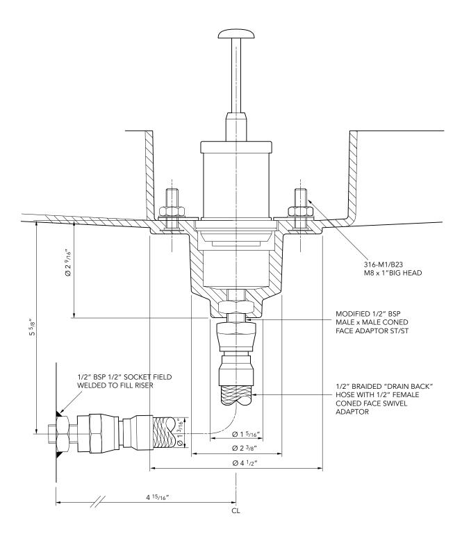
Secondary contained remote fill sump. 23" dia. x 25" deep solid base sump with a sealed secondary spill container with integrated drainback system. 18" dia flat sealed cover and frame. Sealkits included.
