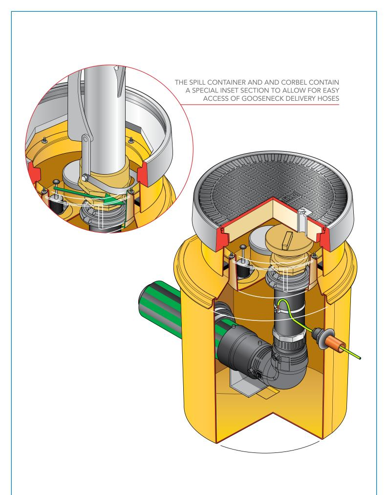
Secondary contained remote fill sump. 23" dia. x 25" deep solid base sump with a sealed secondary spill container with integrated drainback system. 18" dia flat sealed cover and frame. Sealkits included.
