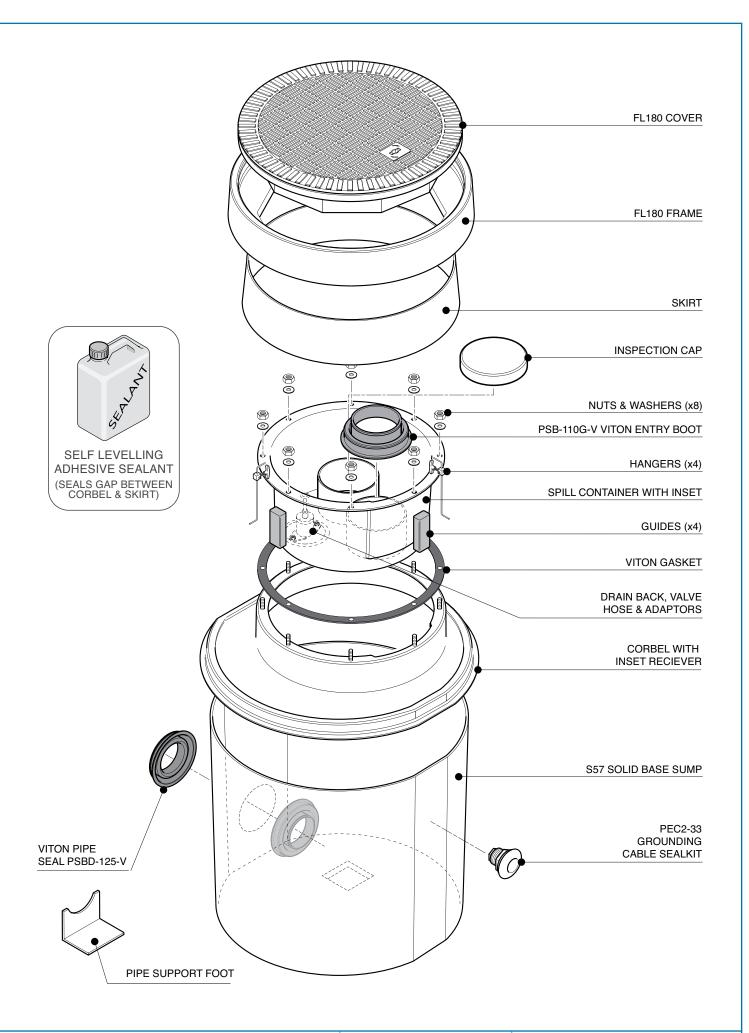
Secondary contained remote fill sump. 23" dia. x 25" deep solid base sump with a sealed secondary spill container with integrated drainback system. 18" dia flat sealed cover and frame. Sealkits included.
