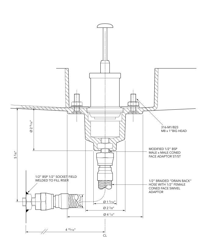
Secondary contained vapour recovery sump. 23" dia. x 25" deep solid base sump with a sealed secondary spill container and integrated drainback system. 18" dia flat sealed cover and frame. Pipework included.
