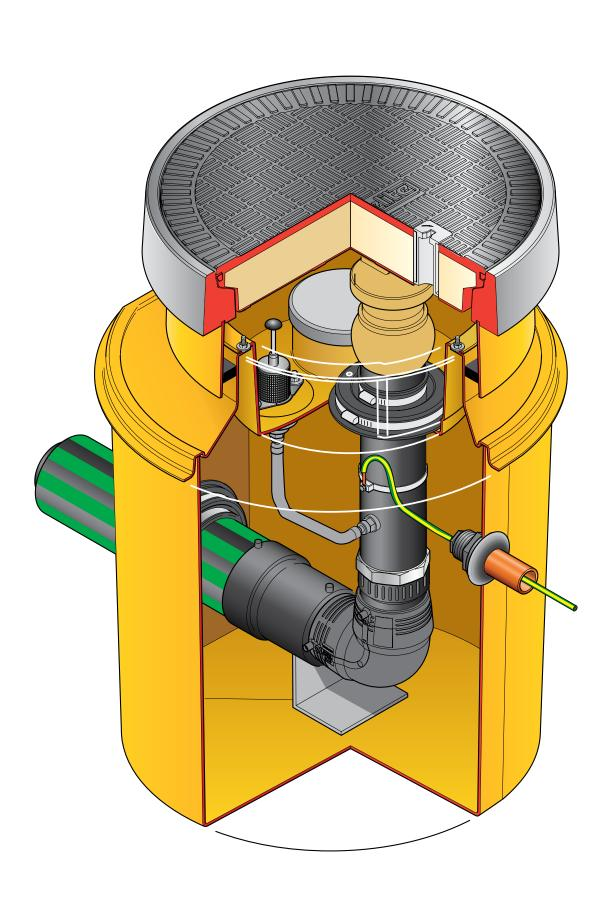
Secondary contained vapour recovery sump. 23" dia. x 25" deep solid base sump with a sealed secondary spill container and integrated drainback system. 18" dia flat sealed cover and frame. Pipework included.
