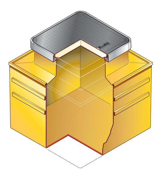
$47\ensuremath{\text{"}}$  square solid base chamber with a corbel and square 30\ensuremath{\text{"}} flat sealed cover.
