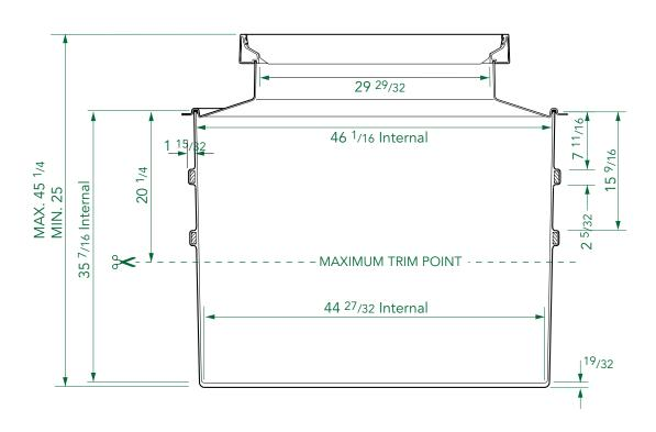
$47\ensuremath{\text{"}}$  square solid base chamber with a corbel and square  $30\ensuremath{\text{"}}$  flat sealed cover.
