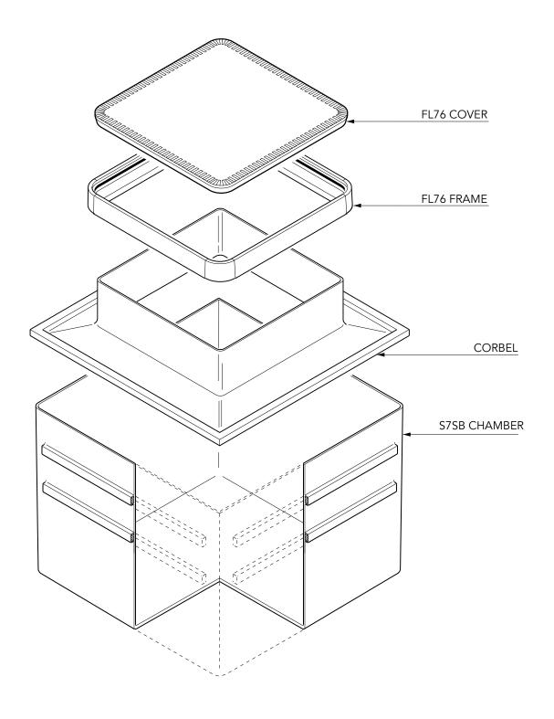
$47\ensuremath{\text{"}}$  square solid base chamber with a corbel and square 30\ensuremath{\text{"}} flat sealed cover.
