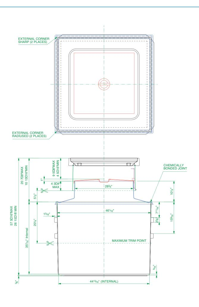
$48\mbox{"}$  square solid base chamber with a corbel, non-structural lid,  $\,$  adjustable skirt, frame and square 30\mbox{"} flat sealed cover.
