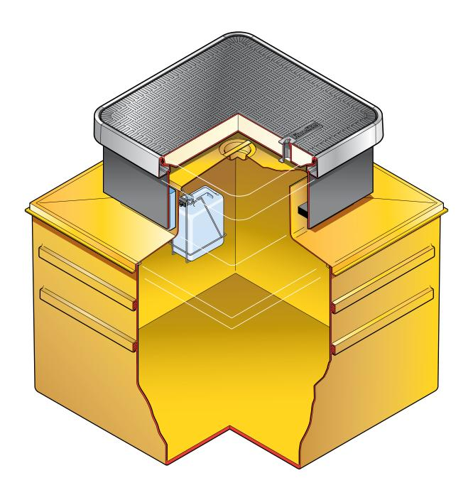
$48\mbox{"}$  square solid base chamber with a corbel, non-structural lid,  $\,$  adjustable skirt, frame and square 30\mbox{"} flat sealed cover.
