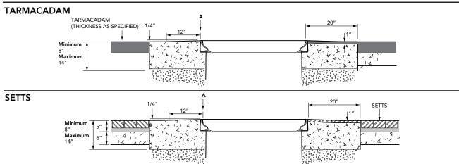
48" square solid base chamber with a corbel, non-structural lid,  $\,$  adjustable skirt, frame and square 30" flat sealed cover.
