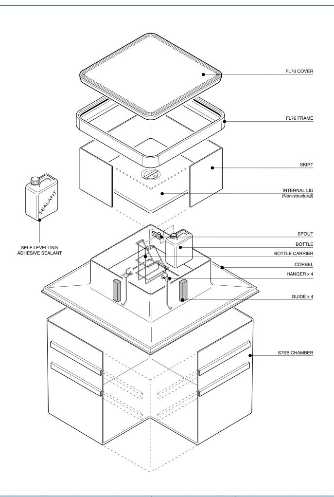
$48\mbox{"}$  square solid base chamber with a corbel, non-structural lid,  $\,$  adjustable skirt, frame and square 30\mbox{"} flat sealed cover.
