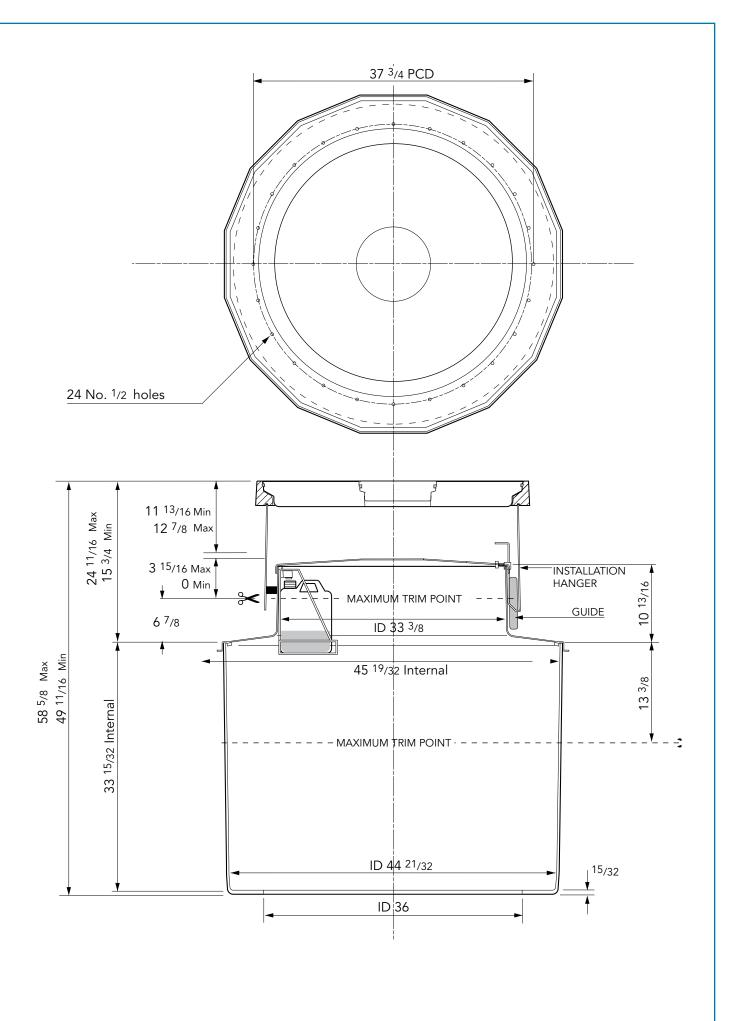
47" diameter bolted base chamber with a corbel, adjustable skirt, non-structural internal lid with a central hole and round 35" flat sealed cover with central manual dip cover. Round tank flange.
