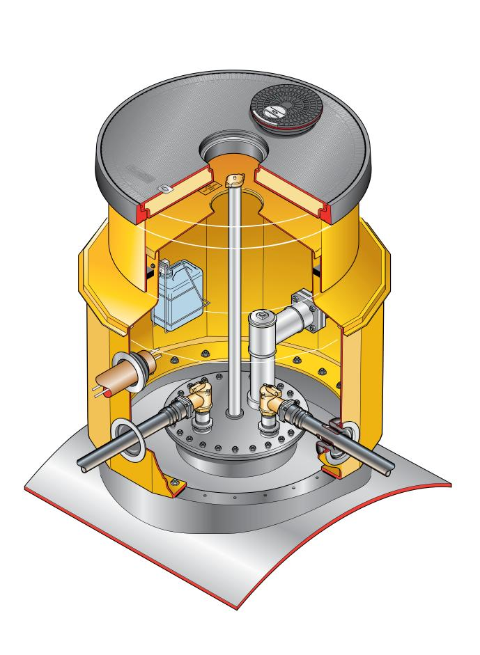
47" diameter bolted base chamber with a corbel, adjustable skirt, non-structural internal lid with a central hole and round 35" flat sealed cover with central manual dip cover. Round tank flange.
