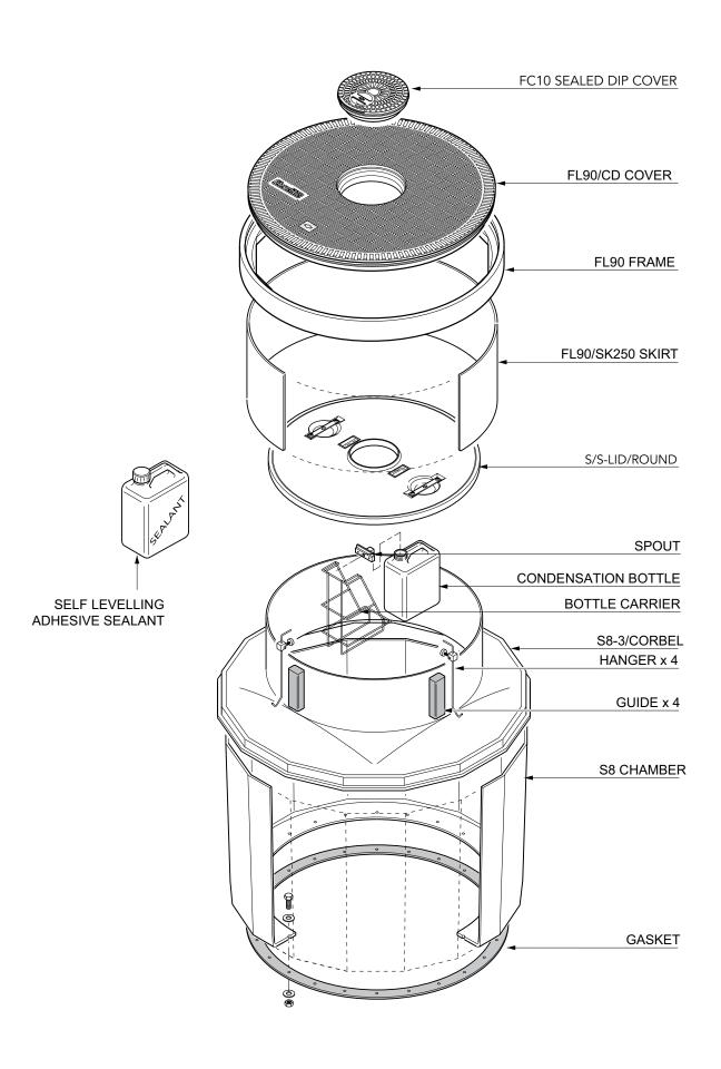
47" diameter bolted base chamber with a corbel, adjustable skirt, non-structural internal lid with a central hole and round 35" flat sealed cover with central manual dip cover. Round tank flange.
