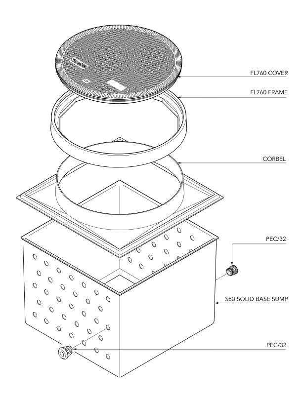
33 15/16" x 33 15/16" x 26 9/16" deep solid base sump with a corbel and 30" dia. flat sealed cover and frame
