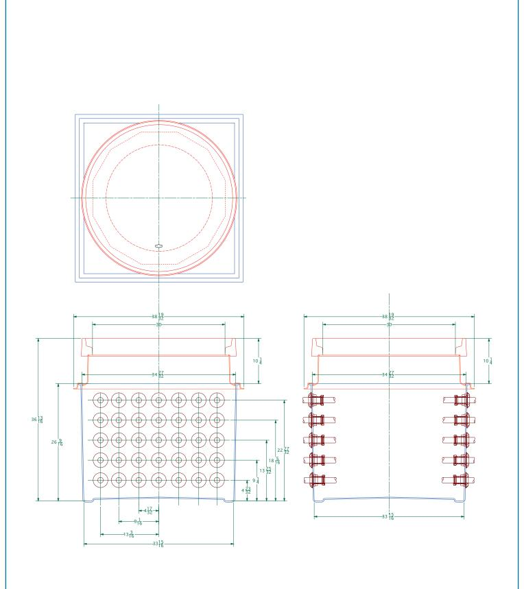
33 15/16" x 33 15/16" x 26 9/16" deep solid base sump with a corbel and 30" dia. flat sealed cover and frame
