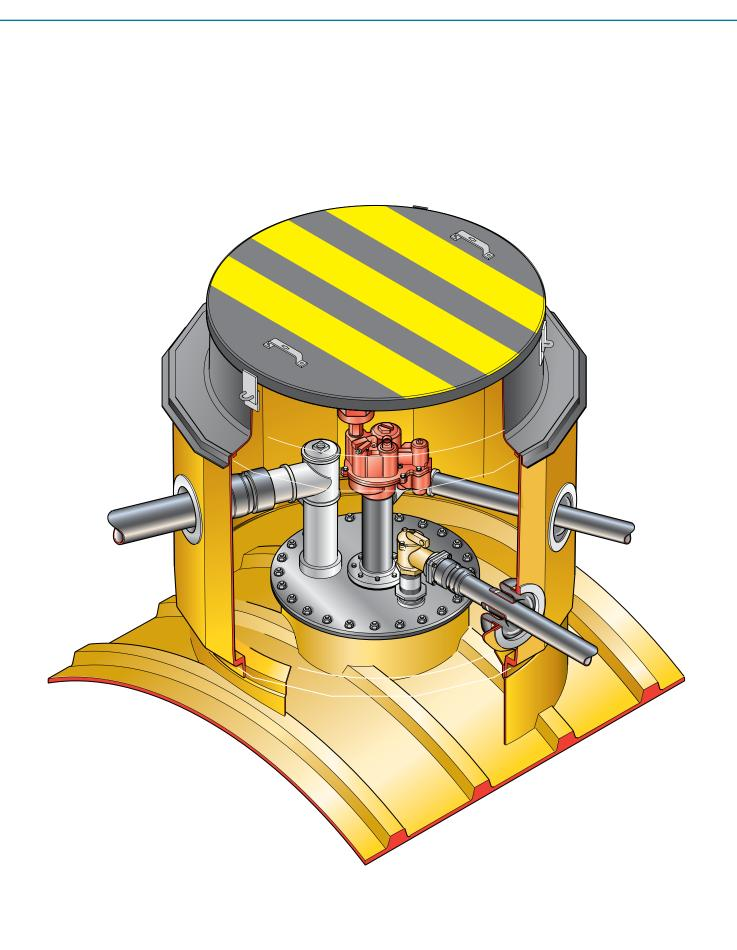
$47^{\circ}$  diameter sump with collar ring base, corbel and lockable lid. Designed for green area applications.
