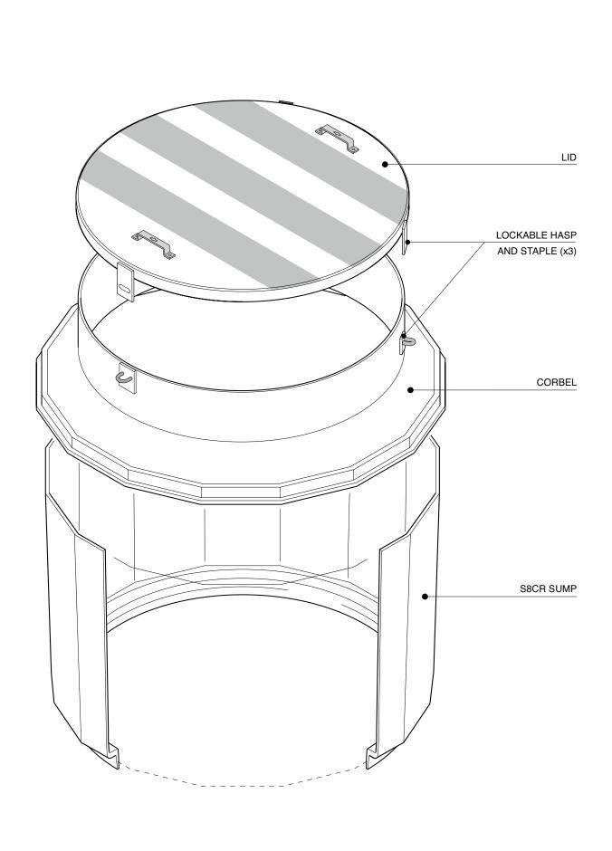
47" diameter sump with collar ring base, corbel and lockable lid. Designed for green area applications.
