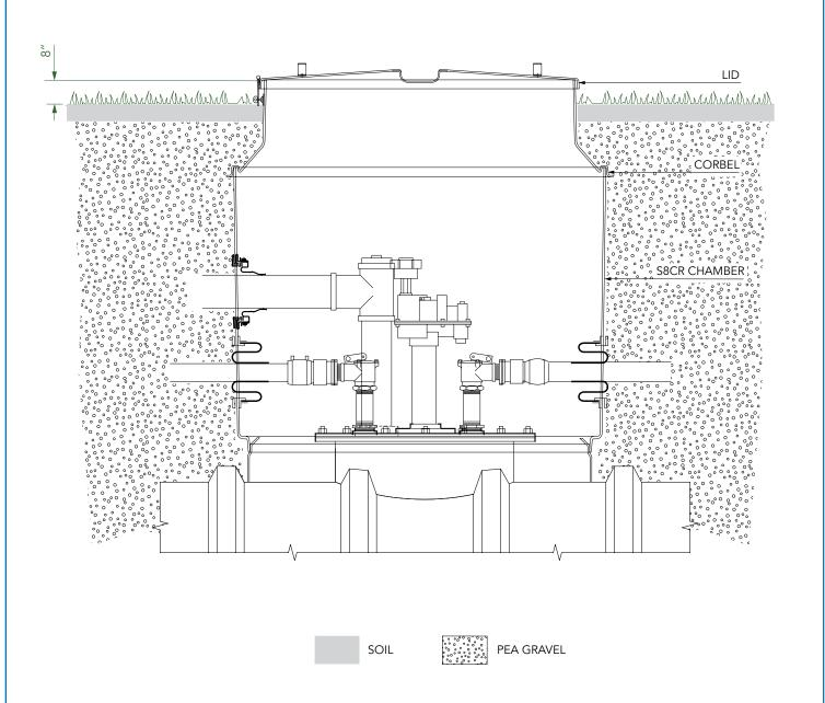
$47^{\circ}$  diameter sump with collar ring base, corbel and lockable lid. Designed for green area applications.
