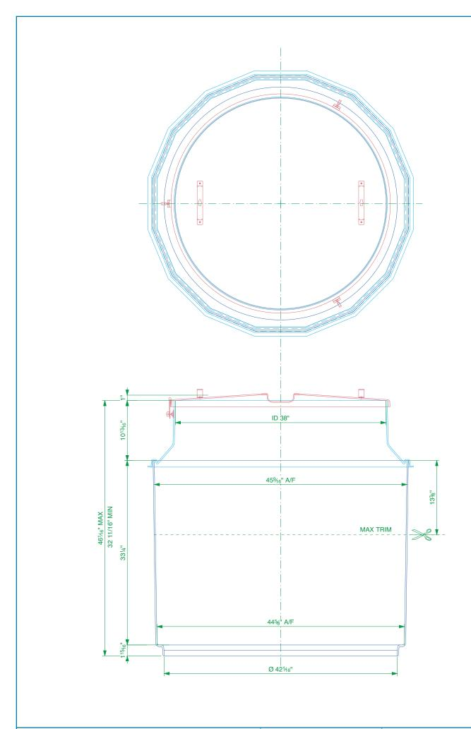
$47^{\circ}$  diameter sump with collar ring base, corbel and lockable lid. Designed for green area applications.
