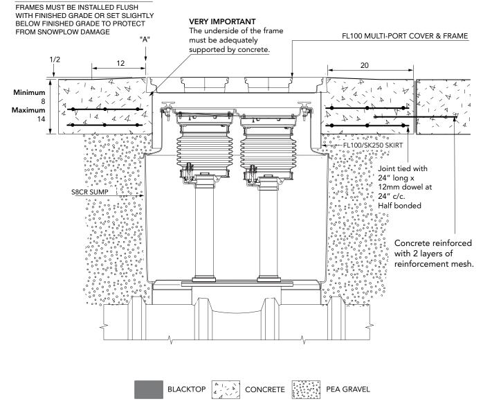
$45^\circ$  diameter x  $33^\circ$  deep sump base to fit  $42^\circ$  tank collar ring, corbel and watertight spill platform for (2) 5-gallon spill buckets.  $36^\circ$  diameter multiport cover, frame and skirt.
