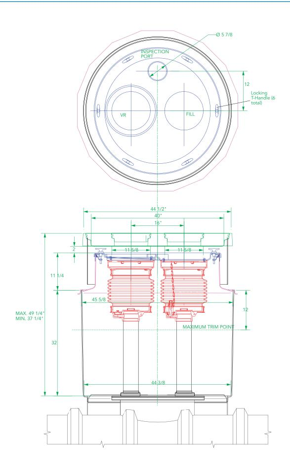
$45^{\circ}$  diameter x 33° deep sump base to fit 42° tank collar ring, corbel and watertight spill platform for (2) 5-gallon spill buckets. 36° diameter multiport cover, frame and skirt.
