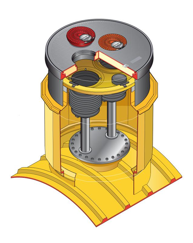
$45^{\circ}$  diameter x 33° deep sump base to fit 42° tank collar ring, corbel and watertight spill platform for (2) 5-gallon spill buckets. 36° diameter multiport cover, frame and skirt.
