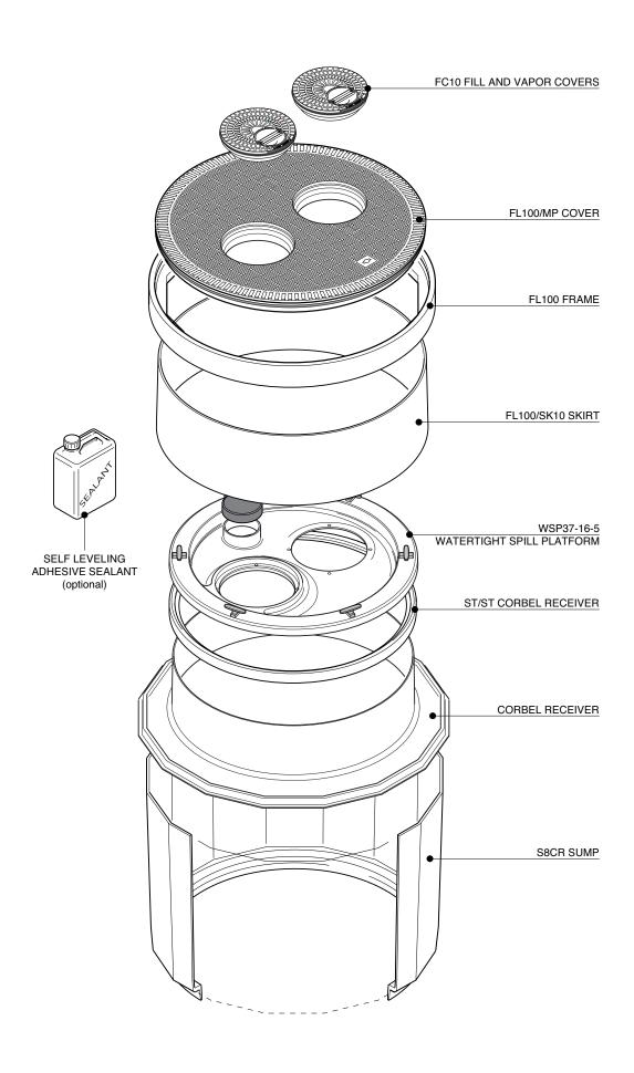
$45^{\circ}$  diameter x 33  $^{\circ}$  deep sump base to fit 42  $^{\circ}$  tank collar ring, corbel and watertight spill platform for (2) 5-gallon spill buckets. 36  $^{\circ}$  diameter multiport cover, frame and skirt.
