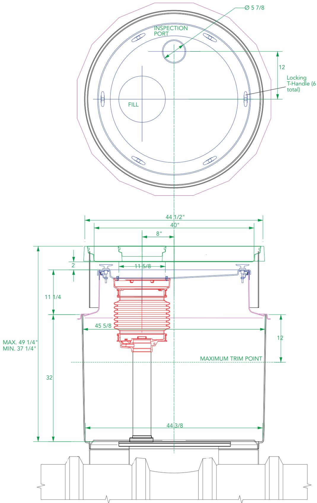
45" diameter x 33" deep sump base to fit 42" tank collar ring, corbel and watertight spill platform for a single 5-gallon spill bucket. 40" diameter offset fill cover, frame and skirt.
