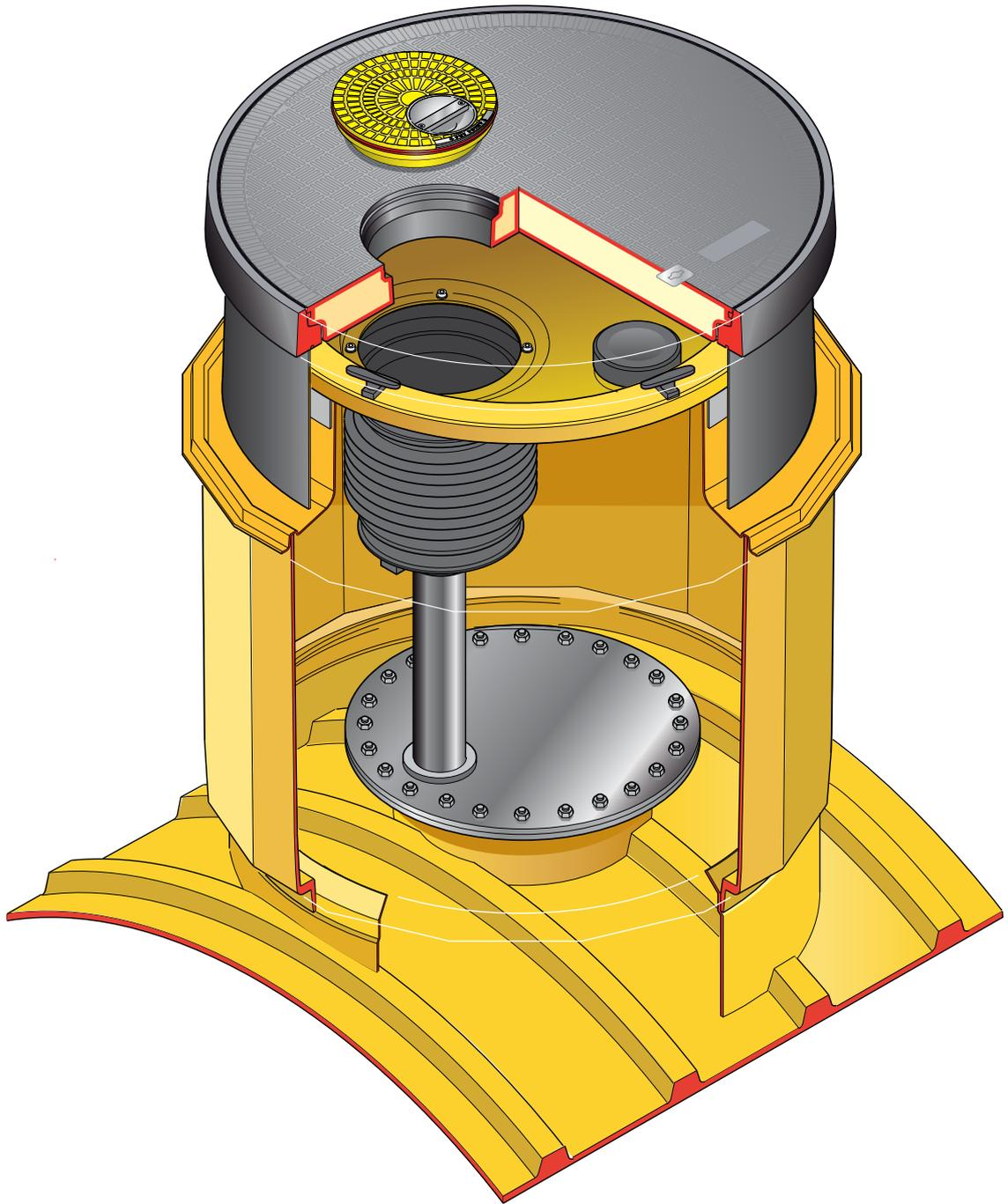
45" diameter x 33" deep sump base to fit 42" tank collar ring, corbel and watertight spill platform for a single 5-gallon spill bucket. 40" diameter offset fill cover, frame and skirt.
