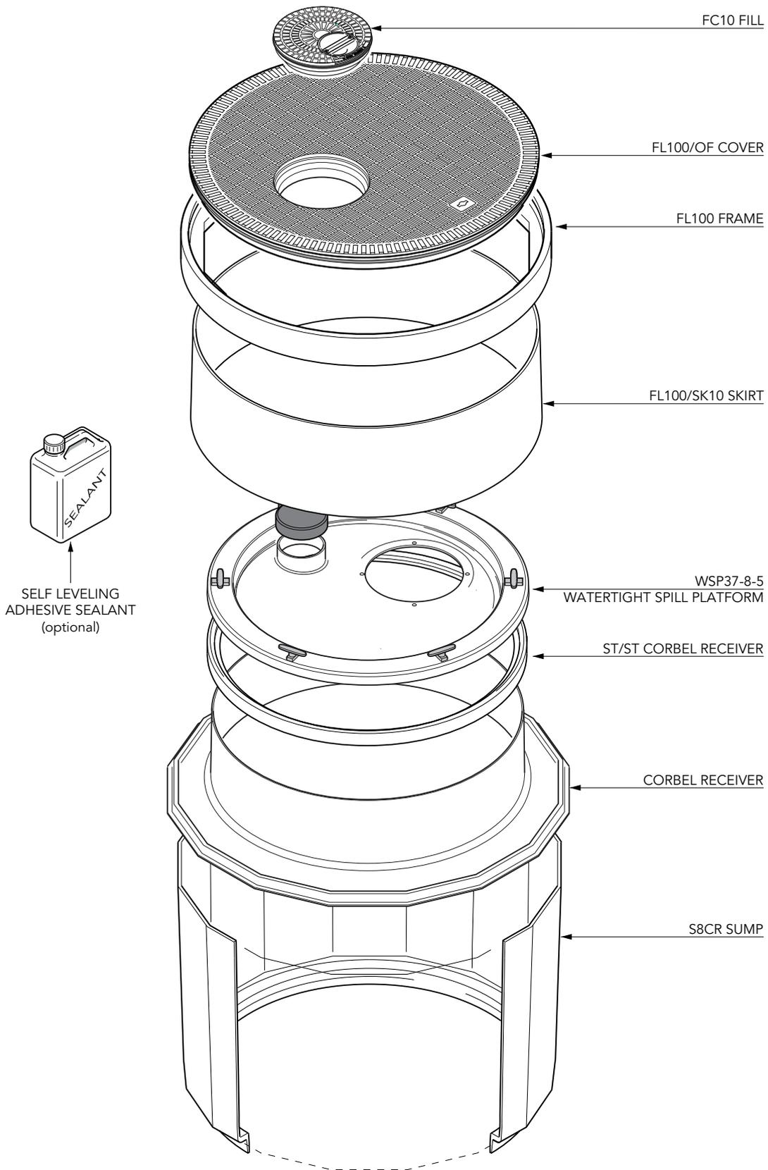
45" diameter x 33" deep sump base to fit 42" tank collar ring, corbel and watertight spill platform for a single 5-gallon spill bucket. 40" diameter offset fill cover, frame and skirt.
