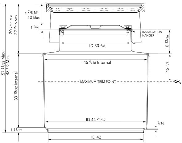
Watertight FRP sumps to fit 42" tank collar with a sealed corbel, watertight inner lid and 42" watertight, flat sealed manhole cover.
