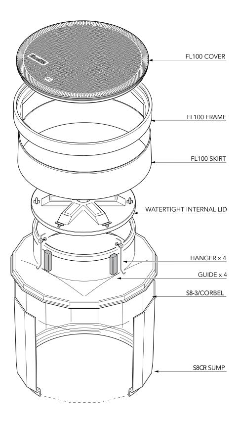
Watertight FRP sumps to fit 42" tank collar with a sealed corbel, watertight inner lid and 42" watertight, flat sealed manhole cover.
