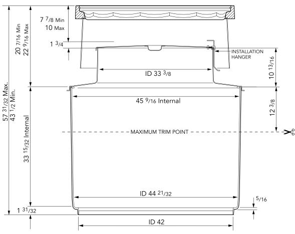
FRP sumps to fit 42" tank collar with a sealed corbel, internal lid and 42" watertight, flat sealed manhole cover.
