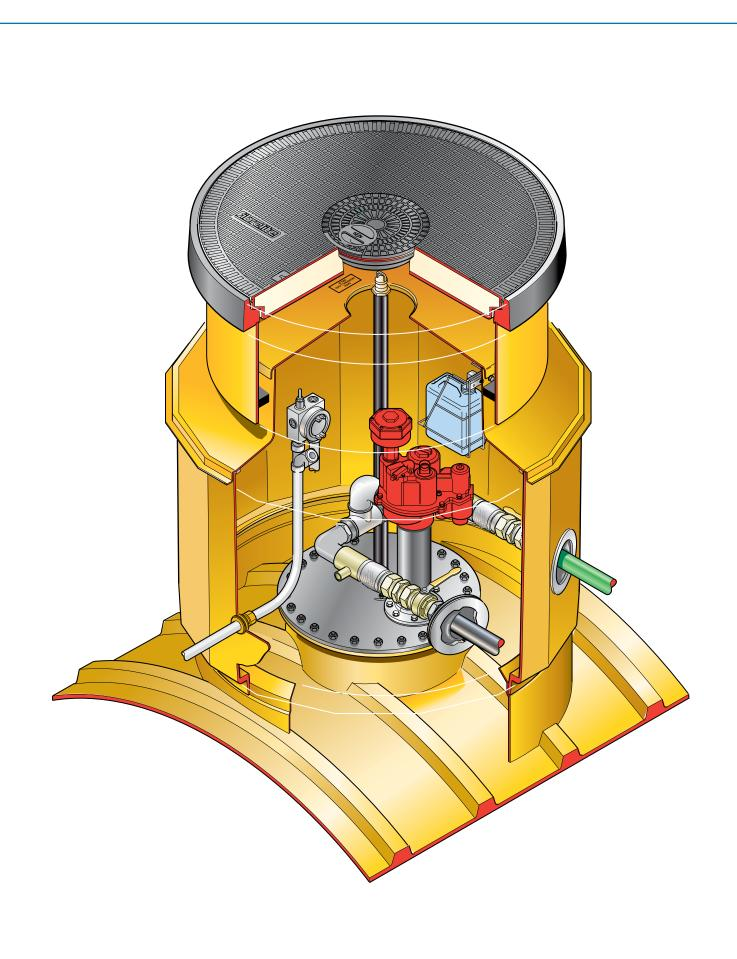
45" diameter sump to fit 42" tank collar ring with corbel, internal lid, adjustable skirt and round 36" central dip flat sealed cover, corbel/skirt sealkit with condensation bottle and fixing kit.
