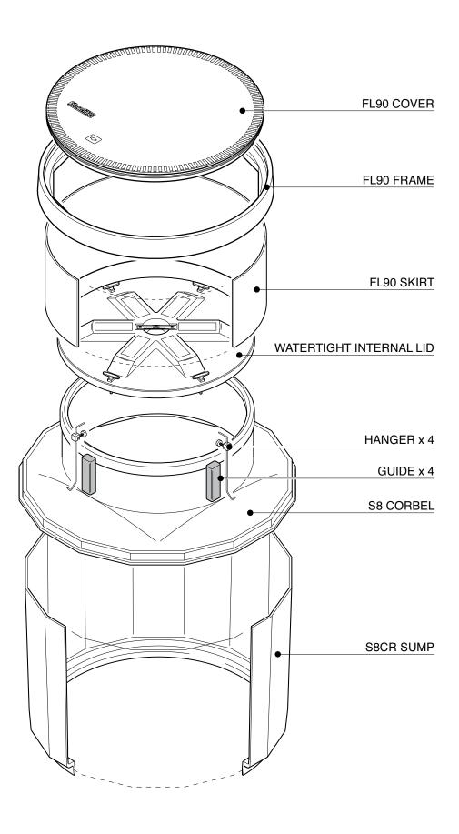
Watertight FRP sumps to fit 42" tank collar, corbel, watertight inner lid and 36" watertight, flat sealed manhole cover.
