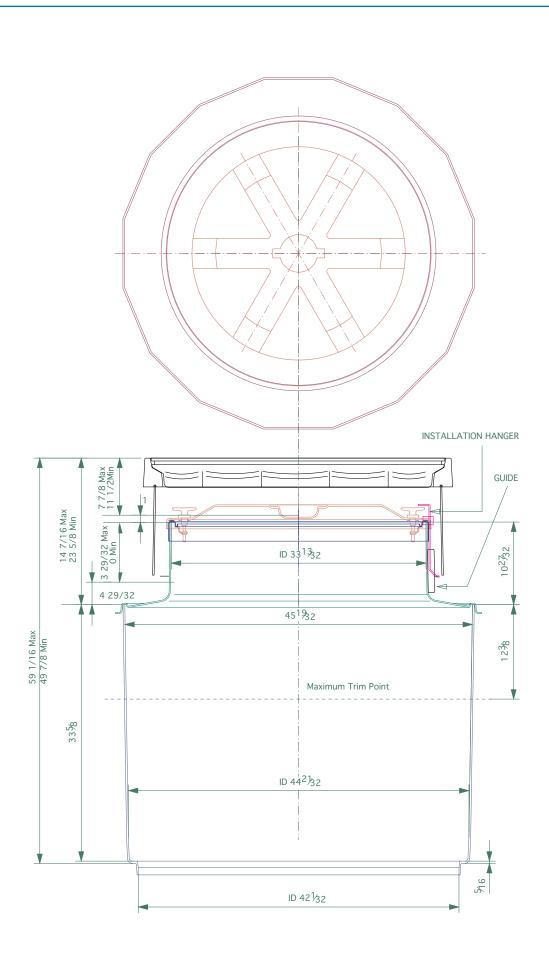
Watertight FRP sumps to fit 42" tank collar, corbel, watertight inner lid and 36" watertight, flat sealed manhole cover.
