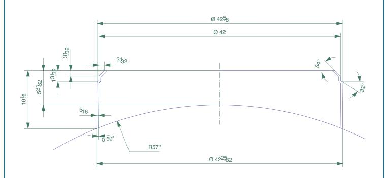
Tank collar to fit S8CR collar ring chamber/sump.
