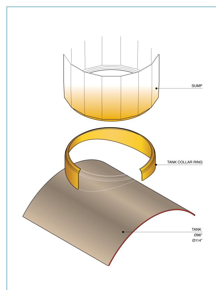
Tank collar to fit S8CR collar ring chamber/sump.
