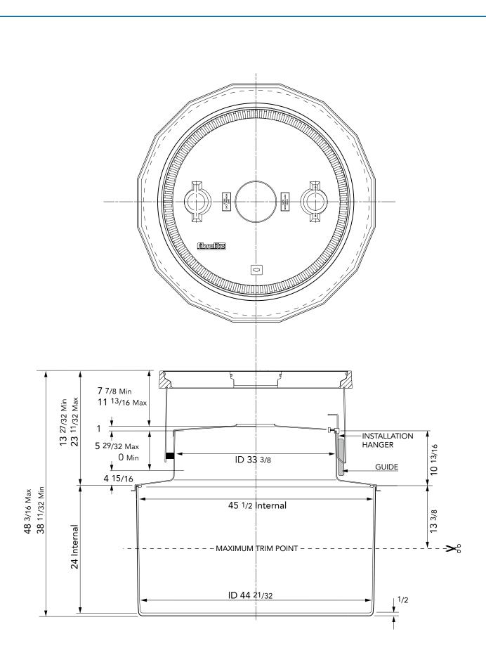
45" diameter base sump with a sealed corbel, internal lid, adjustable skirt, and round 36" flat sealed central dip cover. Structural base. Normal burial.
