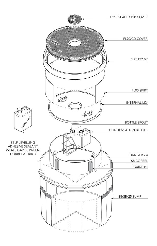
45" diameter base sump with a sealed corbel, internal lid, adjustable skirt, and round 36" flat sealed central dip cover. Structural base.
