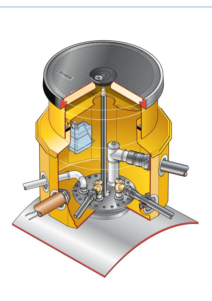
45" diameter base sump with a sealed corbel, internal lid, adjustable skirt, and round 36" flat sealed central dip cover. Structural base.
