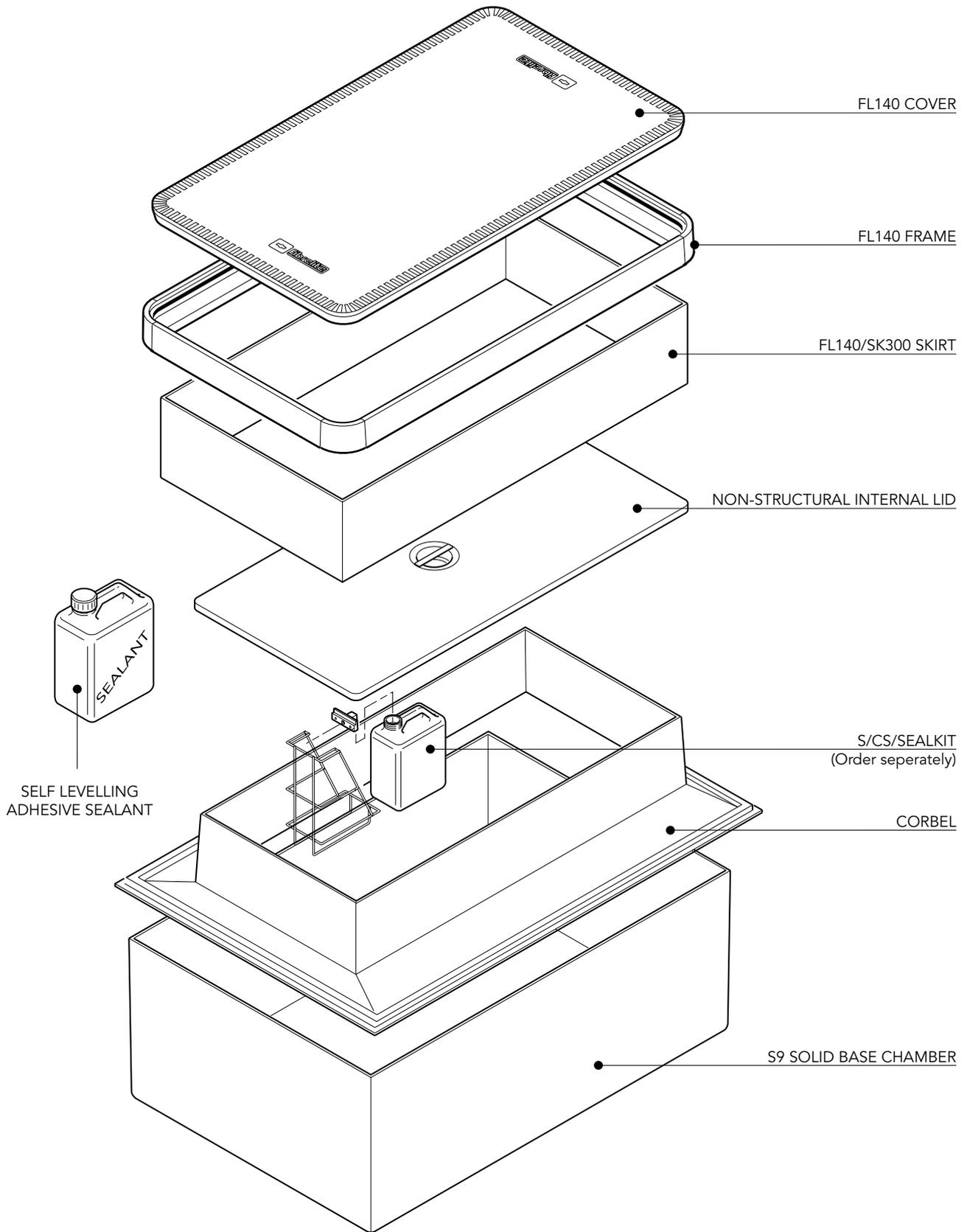
58" x 39" solid base chamber, corbel, adjustable skirt, internal lid and flat sealed cover with frame.
