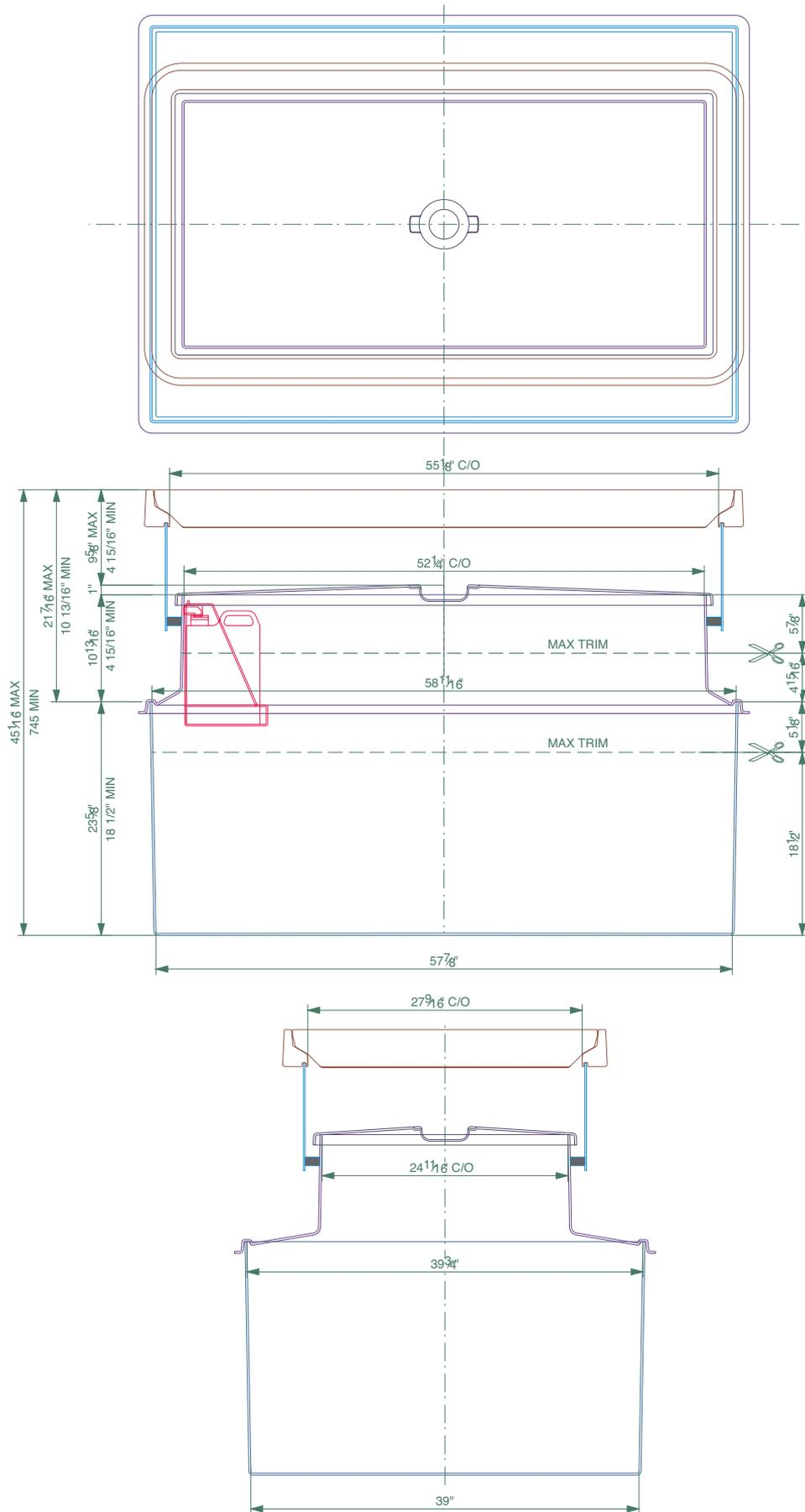
58" x 39" solid base chamber, corbel, adjustable skirt, internal lid and flat sealed cover with frame.
