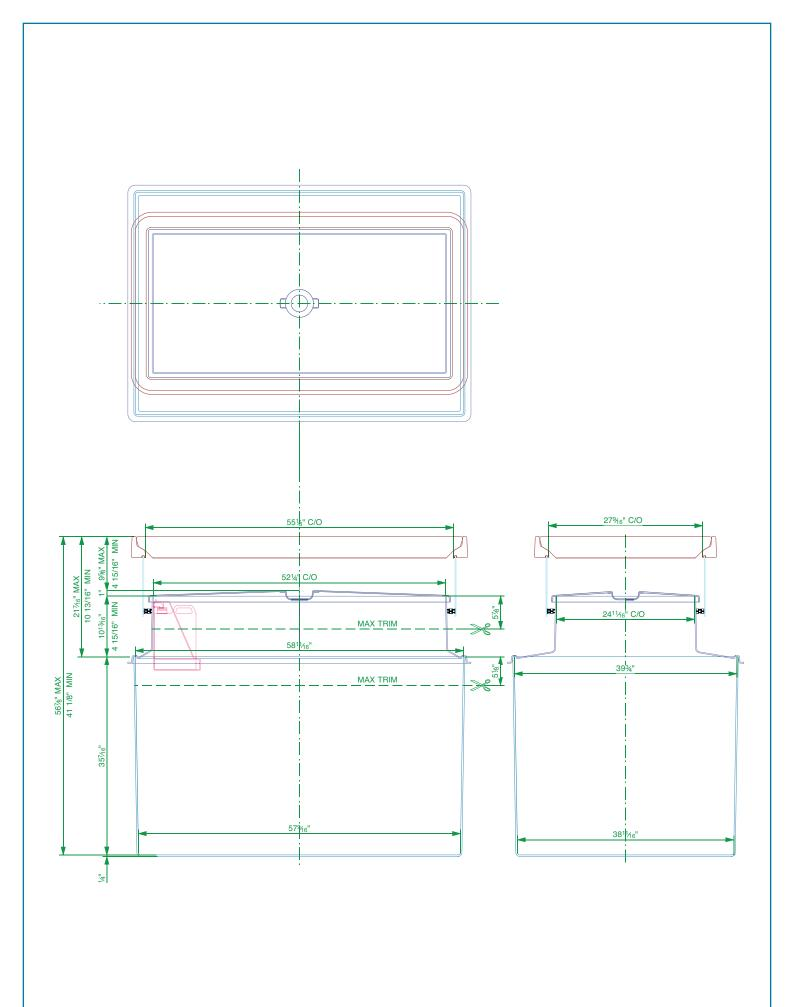
$57~^{9}{\rm /16}^{\circ}$  x  $38~^{11}{\rm /16}^{\circ}$  solid base deep sump, sealed corbel, height adjustable skirt, internal lid, flat sealed cover and frame.
