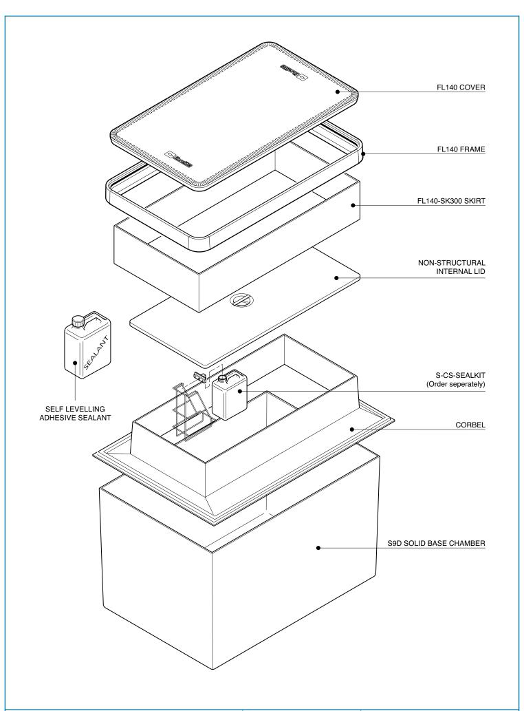
$57\ ^9\text{/16"}$  x 38  $^{11}\text{/16"}$  solid base deep sump, sealed corbel, height adjustable skirt, internal lid, flat sealed cover and frame.
