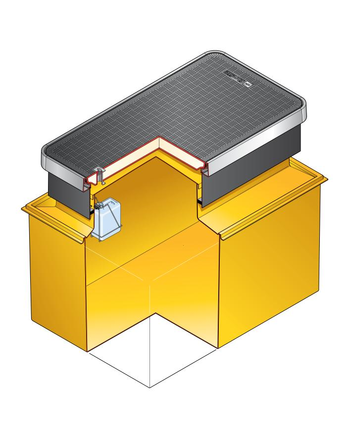
$57~^9/\rm 16^\circ$  x 38  $^{11}/\rm 16^\circ$  solid base deep sump, sealed corbel, height adjustable skirt, internal lid, flat sealed cover and frame.
