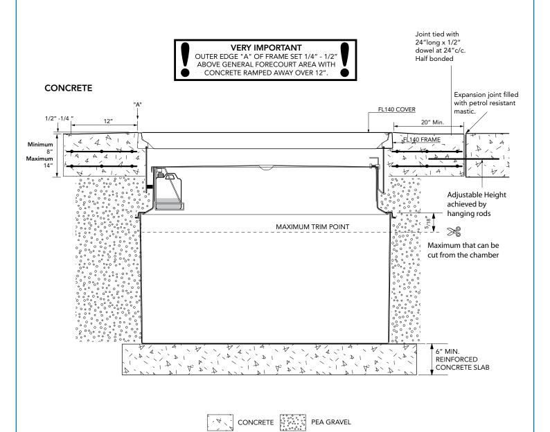
$57~^{9}/16"$  x  $38~^{11}/16"$  solid base deep sump, sealed corbel, height adjustable skirt, internal lid, flat sealed cover and frame.
