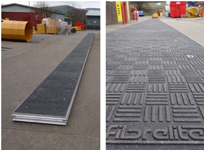
Ensuring a perfect fit, the panels are checked in the encapsulating frame before delivery
