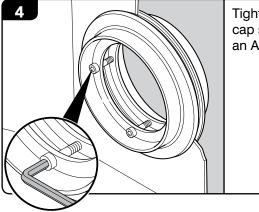
Tighten the socket cap screws with an Allen key.
