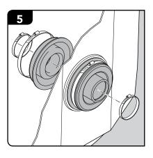
Fit the external entry boot and internal entry boot to the flange rings and secure with the flange ring clips provided.
