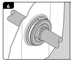
Feed the pipe through the primary bore of the entry boots.
