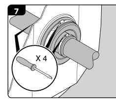
Fit and tighten pipe clips to the entry boots. Clips are to be tightened in accordance with the pipe manufacturers recommendations.
