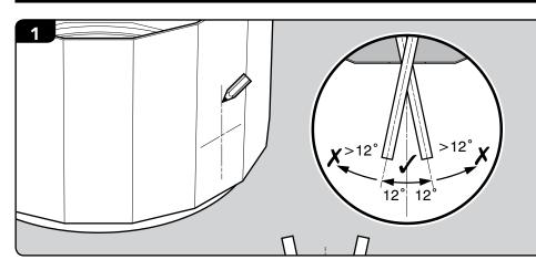
Mark out the lateral and vertical position of the pipe on the sump wall. The exist position of the pipework through the sump wall must be as close as possible to 90 degrees. The angle of the flexible entry sleeve must not exceed 12 degrees from centre line (24 degree inclusive angle)
