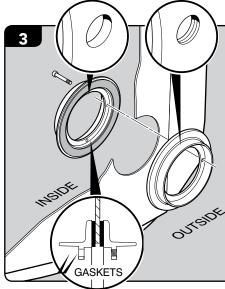
Ensuring that the gaskets are attached to the flange rings, fit the outside flange ring to the outside wall of the sump and the inside flange ring to the inside wall of the sump
