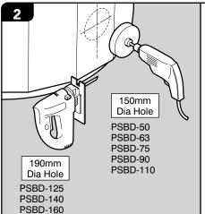
Where appropriate, it is recommended that a drill piloted holesaw be used to cut the pipe seal entry hole in the sump. Where size prohibits the use of a holesaw a jigsaw must be used.
