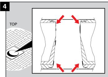
Remove the original adhesive and thoroughly clean the cover flange recesses (top & bottom) and the key housing accommodation hole.
