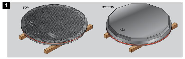
Elevate the cover using wooden blocks to allow the damaged key housing to drop down and protect the cover surface.
