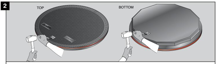
Break either the top or bottom flange of the key-housing away using a cold chisel and hammer
