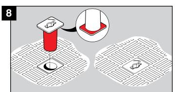
Apply a continuous film of adhesive to the contact surfaces of the key housing. Insert the key housing into the cover, locating the key housing flange in the cover top flange recess.
