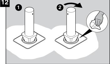
Insert the Swaging Punch into the bore of the retainer and strike with hammer; turn the Swaging Punch through approx 45° and strike again to achieve an additional mechanical bond. Remove excessive adhesive.
