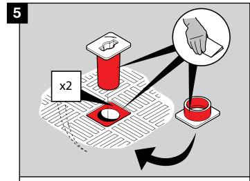
Using the sand paper, abrade the contact surfaces of the key housing and retainer. Also abrade the cover flange recesses.
