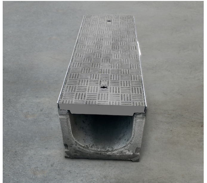
Covers were stepped from 40 to 65mm deep to meet E600 load rating
